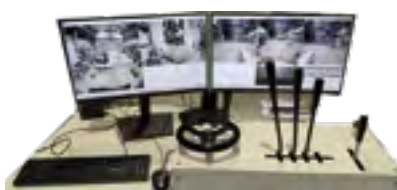
Remote forklift-specific interface that allows intuitive operation of driving and cargo handling using wide-angle camera video and augmented reality guide lines
