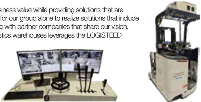
Remote forklift-specific interface that allows intuitive operation of driving and cargo handling using wide-angle camera video and augmented reality guide lines
