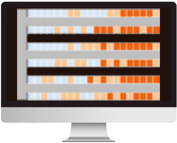
Visualizing congestion status by coloring each chute based on volume
